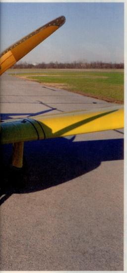
Many Ercoupe owners replace the stock metal propellers with Sensenich wood propellers (above left) to gain about 40 pounds of useful load. Vacuum for this model 415-C's heading indicator is supplied by ram air passing through a fuselage-mounted venturi tube (top right). Vintage touches include a master switch mounted behind the passenger seat and navigation lights secured by wire balls (above right).
